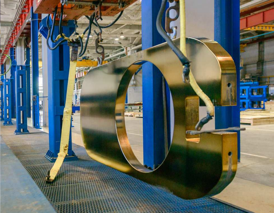
Nickel-plating line with application of silicon carbide nanoparticles according to the technologies of Kanigen (Japan) was launched in 2015
