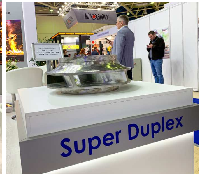
The super duplex impeller for the fire pump. KONAR introduced a technological process within the framework of R&D confirming its high competencies.
