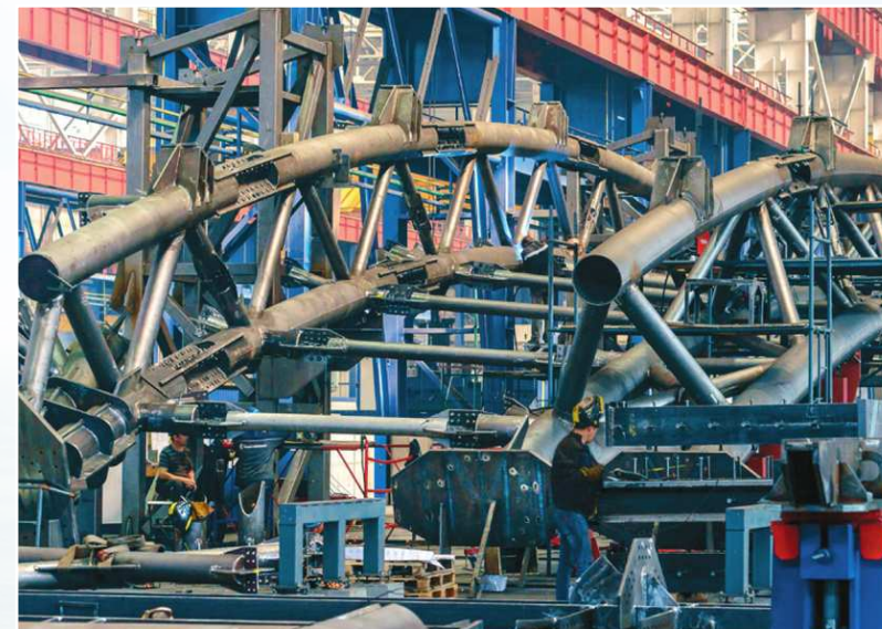
Preliminary assembly of the arch for Lakhta Center was performed in the workshop of JV KONAR-Cimolai
