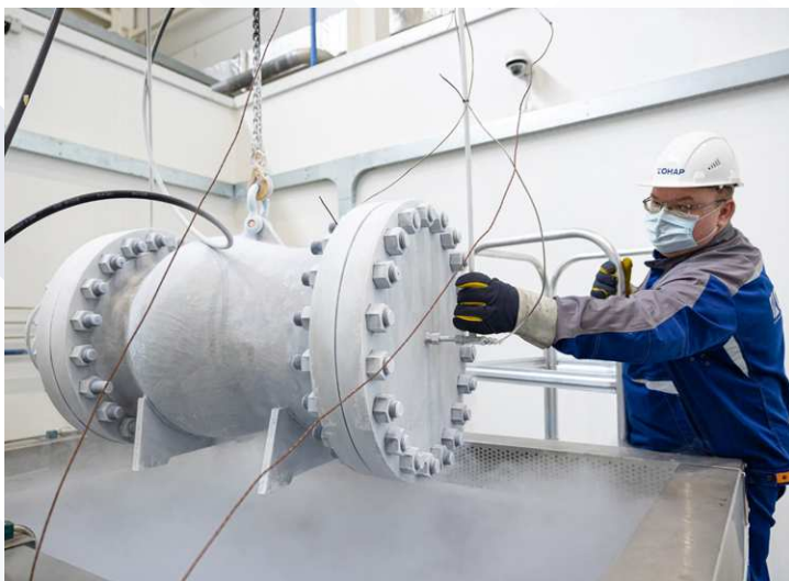
Cryogenic testing at -196^{\circ}\text{C}
