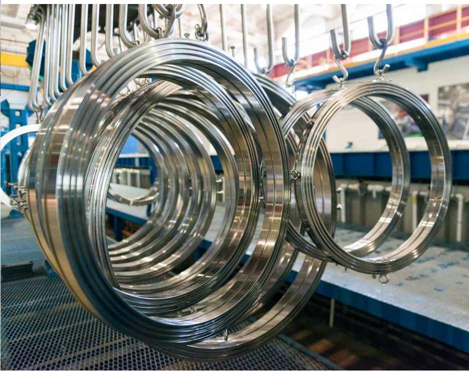
Nickel-plating line with application of silicon carbide nanoparticles according to the technologies of Kanigen (Japan) was launched in 2015
