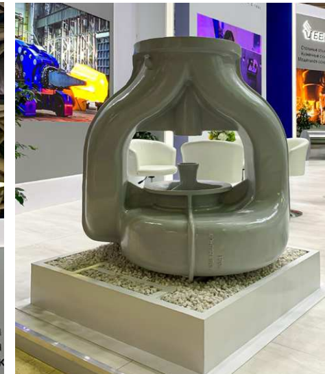
Complex casting – volute of the pump НПВ 1250
